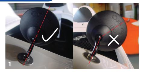
Adjust the mirror before dismounting it, adjustment will be limited after the cone is glued on.
